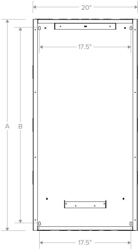
Surface Mount Panel Dimensions
