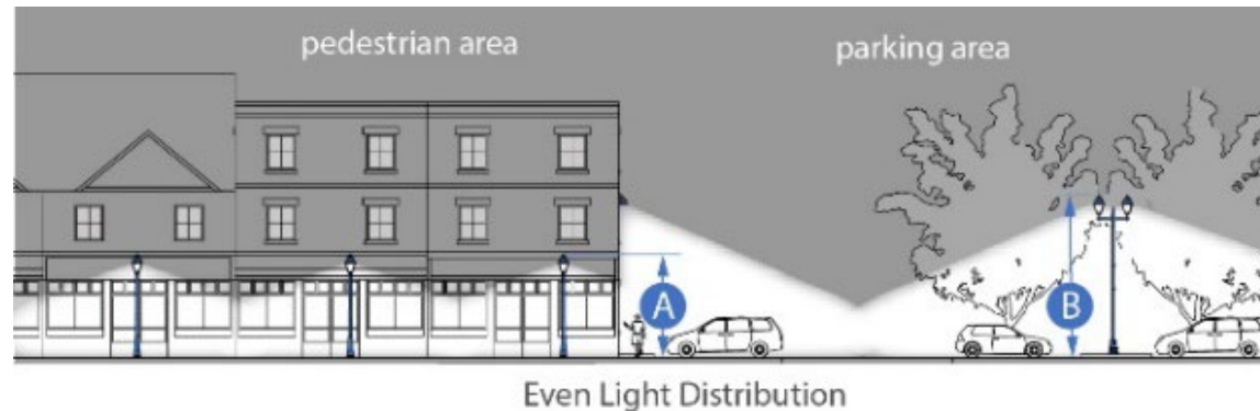
Figure 101. Illustration showing the use of multiple low powered light fixtures to produce pedestrian scale lighting with even distribution.
